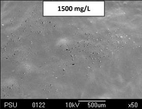
Figure 7. Scanning electron micrograph of edible HPMC films containing 900 mg/L and 1500 mg/L phayom wood extract.
